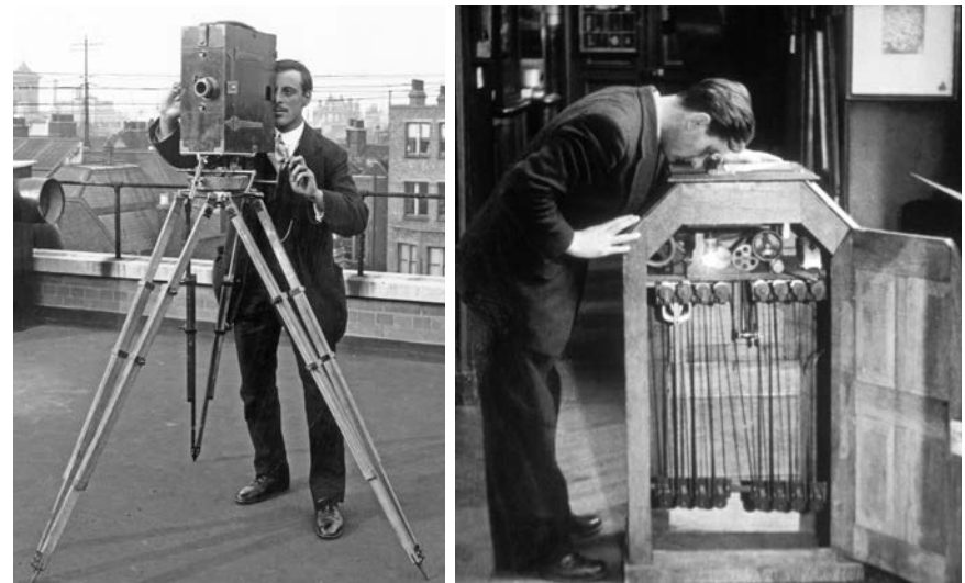
Edison's movie camera (left) and his machine that showed movies (right)
